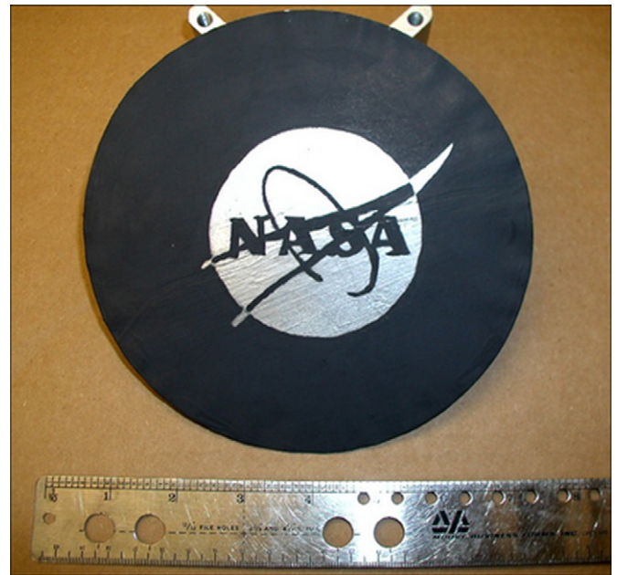
Fig. 7. Large area (285 cm 2 active area) YSZ-based BSC fabricated at 1400 °C.
